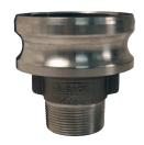
NOTE: In jump size couplings, the cam & groove end is the first size given in the part number. (i.e., a 4030-C-AL is a 4" coupler to a 3" hose shank).
