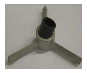
Replace the Teflon® bushing (pos.5) in the spindle steering with a new one.
