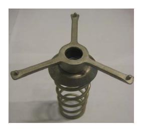
Replace the spring (pos.7), spring cap (pos.6) and the spindle steering (pos.4).
