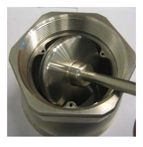
To insert the piston back again it should be putted in a relaxing position in the valve seat
