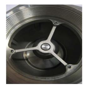
Make sure that the spindle steering is in it's right position.
