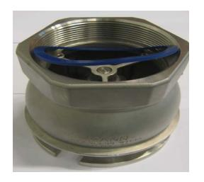
Remove the flat sealing.
